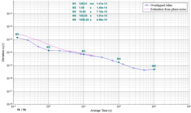
5 MHz / 60min measurement time Residual Overlapped Allan cross variance Deviation ENBW=5Hz
