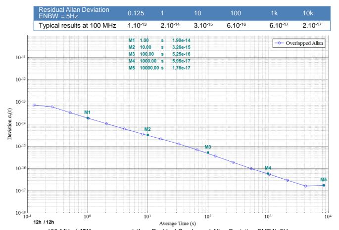
100 MHz / **12H measurement time** Residual Overlapped Allan Deviation ENBW=5Hz
