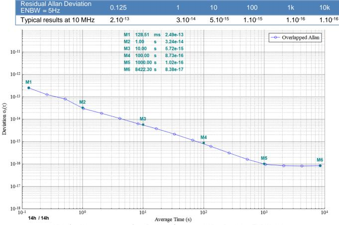
10 MHz / 14H measurement time Residual Overlapped Allan Deviation ENBW=5Hz
